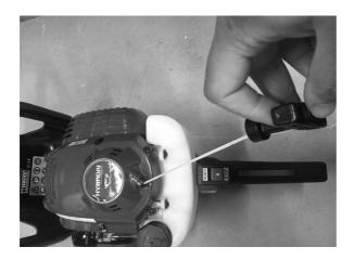
If engine starting is not obtained, put the choke lever on the position and pull again the recoil handle 4 or 5 times and until the tool starts.
